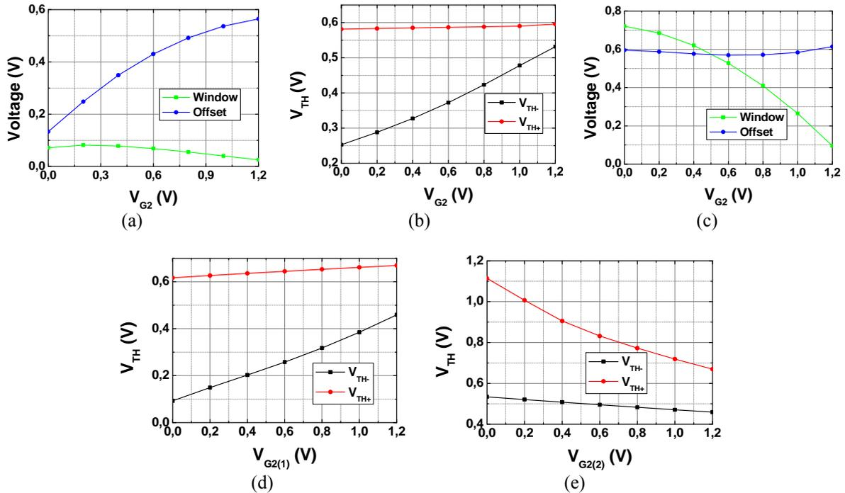
Figure 7. Simulations of the Schmitt triggers based on DCG-FGT transistor
