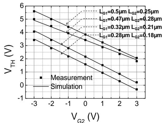
Figure 2. Measured and calculated threshold voltage values versus  $V_{G2}$  for different length ratio configurations
