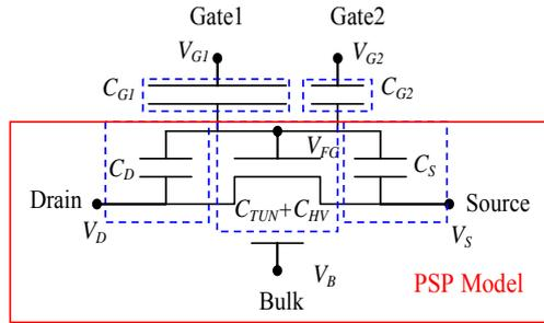
Figure 3. Electrical equivalent circuit of DCG-FGT transistor.
