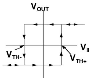
Figure 5. Characteristic of Traditionnal electric scheme of Schmitt trigger.
