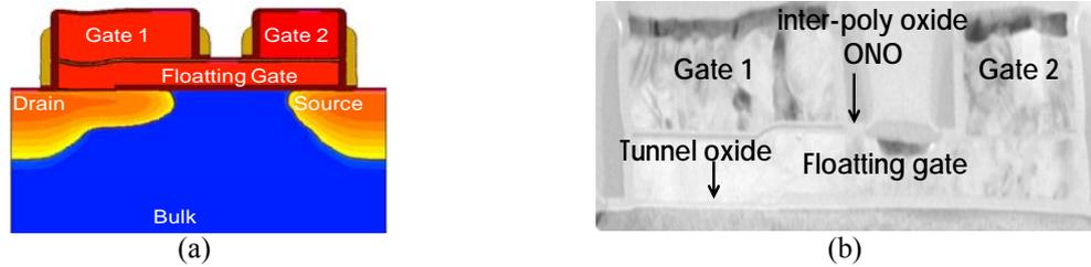
Figure 1. (a) DCG-FGT architecture, (b) Cross section view of a DCG-FGT
