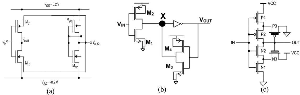
Figure 4. Traditionnal electric scheme of Schmitt trigger.
