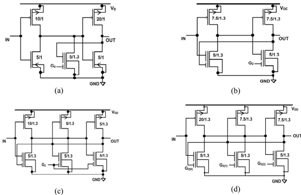
Figure 6. Electrical Scheme of Schmitt Trigger based on DCG-FGT.
